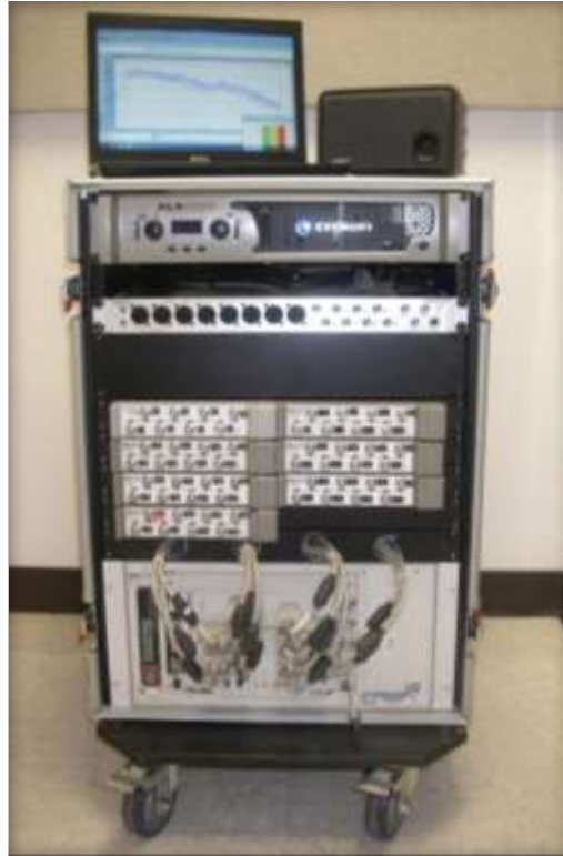
Figure 3.7 A portable dynamic signal analysis system with several input and output channels, a power amplifier, a loudspeaker for monitoring, and a software package.
